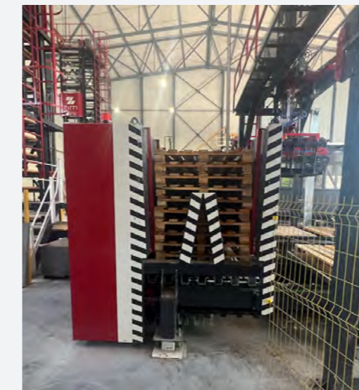
EURO PALLET ROBOT & STACKING EXIT BAND EURO PALET ROBOTU & İSTİF ÇIKIŞ BANDI
